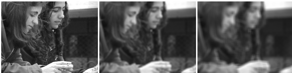
Figure 4.1: Planar isotropic diffusion. Left: original image. Middle and Right: increasing number of diffusion steps.
