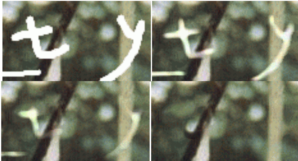
Figure 3.15: Progressive nature of the algorithm. Several intermediate steps of the inpainting of figure 3.12 are shown.
