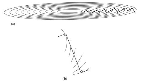
Figure 10.6.1. (a) Steepest descent method in a long, narrow "valley." While more efficient than the strategy of Figure 10.5.1, steepest descent is nonetheless an inefficient strategy, taking many steps to reach the valley floor. (b) Magnified view of one step: A step starts off in the local gradient direction, perpendicular to the contour lines, and traverses a straight line until a local minimum is reached, where the traverse is parallel to the local contour lines.
